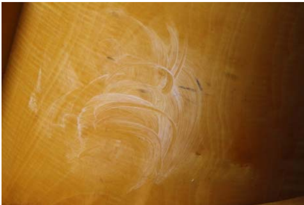
Apply polishing agent to affected area and remove stain. Wait briefly and polish again.
